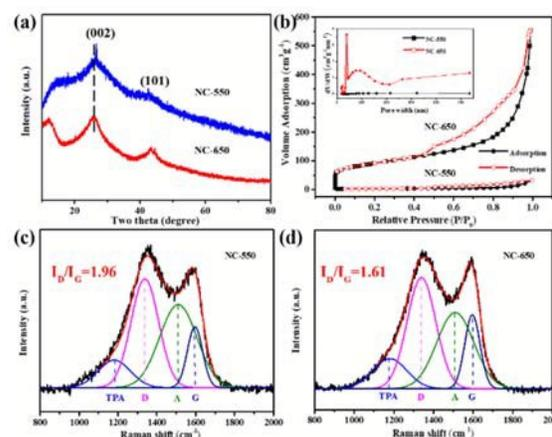
**Fig. 2** (a) XRD data of NC-550 and NC-650; (b)  $\text{N}_2$  adsorption/desorption isotherms of NC-550 and NC-650; Raman spectra of NC-550 (c) and NC-650 (d), which are fitted into four Lorentzian peaks.
