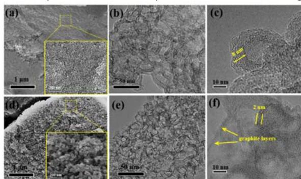
**Fig. 1** SEM and images of NC-550 (a) and NC-650 (d); TEM images of NC-550 (b, c) and NC-650 (e, f).
